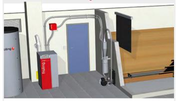
The Froling suction screw system is the ideal solution for rectangular rooms with front-end removal.
