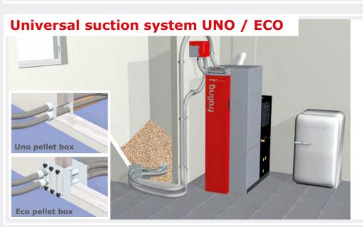
The suction system can handle even large distances between the store and the boiler room. The position of the suction probes and the transfer unit can be adjusted to suit the individual store conditions. The changeover between suction probes is manual **(Eco pellet box)**. There is also a version of the suction system specially for square rooms with an individual probe **(Uno pellet box)**.
