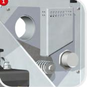
When fuel is fed from the store to the pellet container, the store gate valve opens. The gate valve for the burner closes simultaneously.
